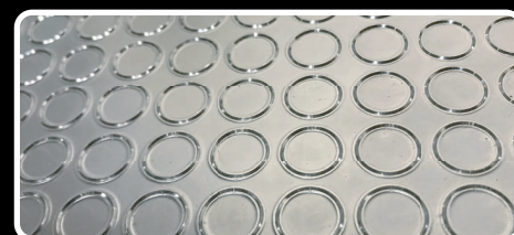
Lower: Flexible dies produced via CNC engraving machines that are capable of intricate patterns and multiple blade heights.
