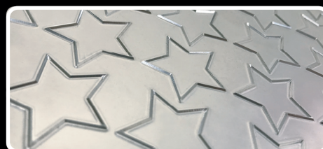
Lower: Flexible dies produced via CNC engraving machines that are capable of intricate patterns and multiple blade heights.
