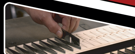
Upper: Steel Rule dies produced by pre-bent metal cutting blades being inserted into notches cut into a wooden base.
