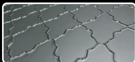
Lower: Flexible dies produced via CNC engraving machines that are capable of intricate patterns and multiple blade heights.
